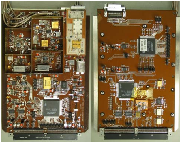
Figure 3- Photographs of Uplink Card
